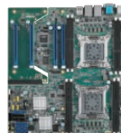
ASMB-920IR Dual Xeon server class EEB MB with dual PCIe x 16, PME expansion, dual-LANs & IPMI
