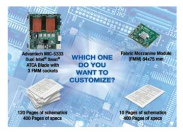
The FMM specification defines the high speed interfaces and associated FRU management. In addition the specification supports a zone 2 connector interface for custom fabric connectivity like SRIO. Signal integrity between FMMs and the Fabric Interface on ATCA blades is ensured via a re-driver between the zone 2 connector and the FMM. A FRU EEPROM on the FMM describes its thermal & power requirements and zone 2 interface information, while all other aspects are managed by a BMC on the ATCA blade.
