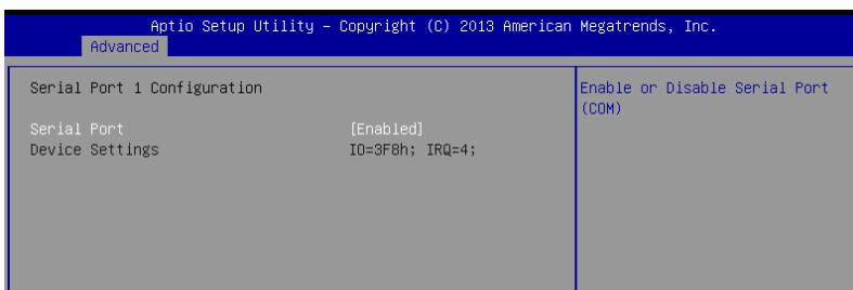
This option enables/disables Serial Ports 1-3, which have fixed I/O port addresses and IRQs: Port1: IO=3F8, IRQ=4, Port2: IO=2F8, IRQ=3, Port3: IO=3E8, IRQ=5.
