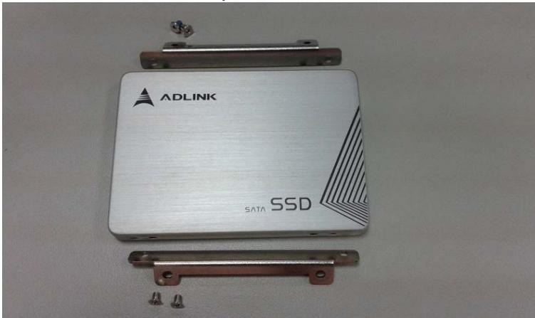
3. Screw the brackets to the 2.5" SATA drive with the four with M3 screws provided.
