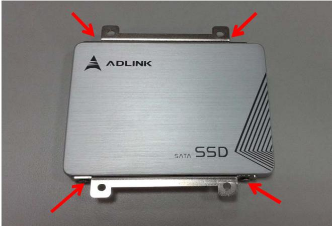
4. Align the drive assembly with the cPCI-3620D/T and insert it into the onboard SATA connector until it is properly seated.
