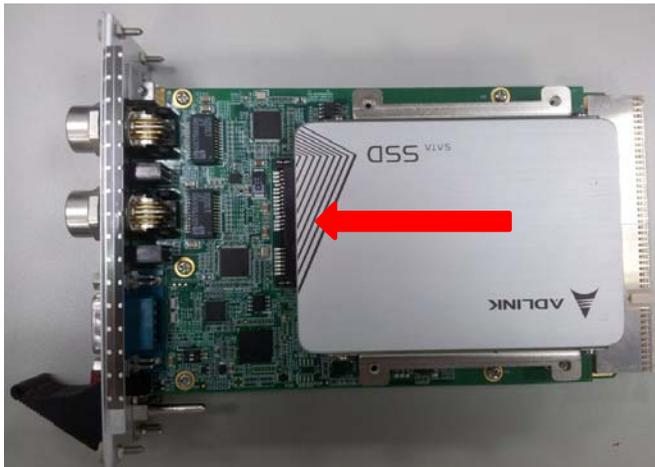
5. Secure the hard drive assembly to the cPCI-3620D/T with four M2.5 screws provided.
