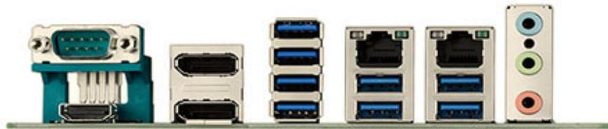
**Figure 1.2 I/O Connectors**
