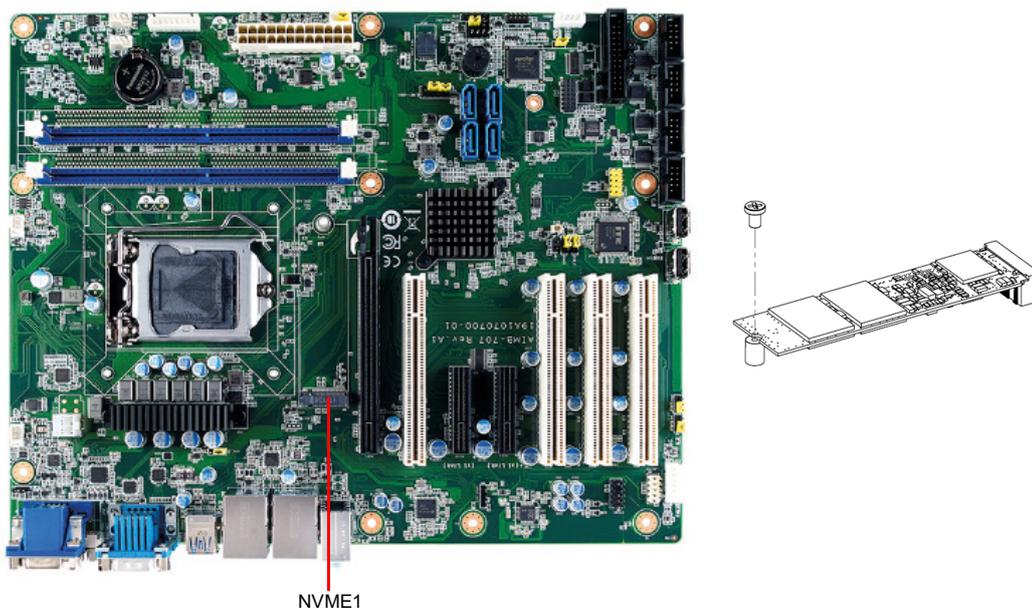
The AIMB-707 G2 sku is equipped with one M.2 socket to support up to PCIe x2 M-key 2280 type storage devices. A screw to fasten the device is already installed on the nut.
