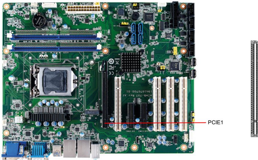
The AIMB-707 provides a PCIe x16 slot for users to install an add-on peripheral card for extension requirements.
