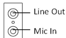
Line Out can be connected to external audio devices like speakers or headphones. Mic In can be connected to a microphone.
