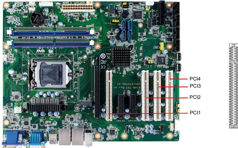
The AIMB-707 provides four 32-bit / 33 MHz PCI slots.
