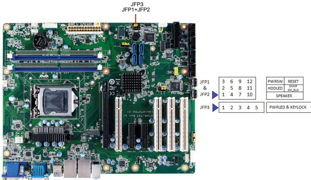
There are several external switches and LEDs to monitor and control the AIMB-707.
