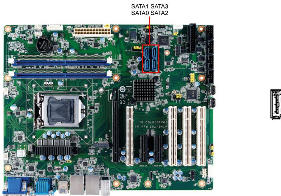
AIMB-707 features four high performance serial ATA 3.0 interfaces (up to 600 MB/s) with long, thin, easy-to-run SATA cables.
