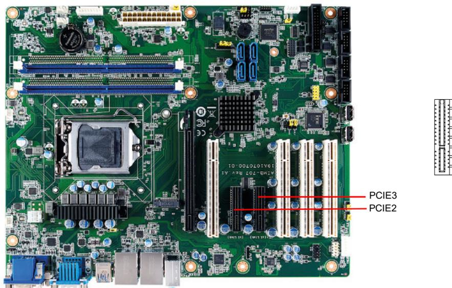
The AIMB-707 offers two PCIe x4 slots for users to install add-on cards for extension requirements. PCIE2 and PCIE3 are PCIe x1 link.
