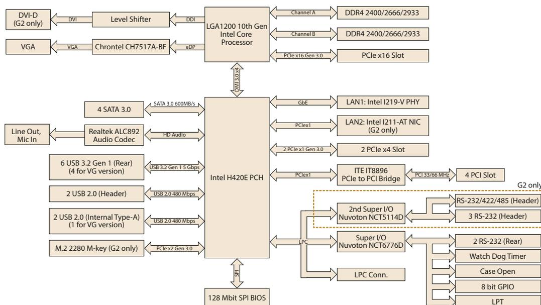
Figure 1.3 Block Diagram
