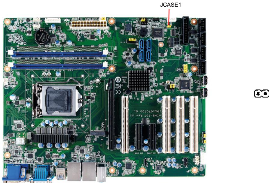
JCASE1 is for chassis with a case open sensor. The buzzer on the motherboard sounds if the case is opened unexpectedly. The default function is disabled and pins 1-2 is bridged by a jumper cap.
