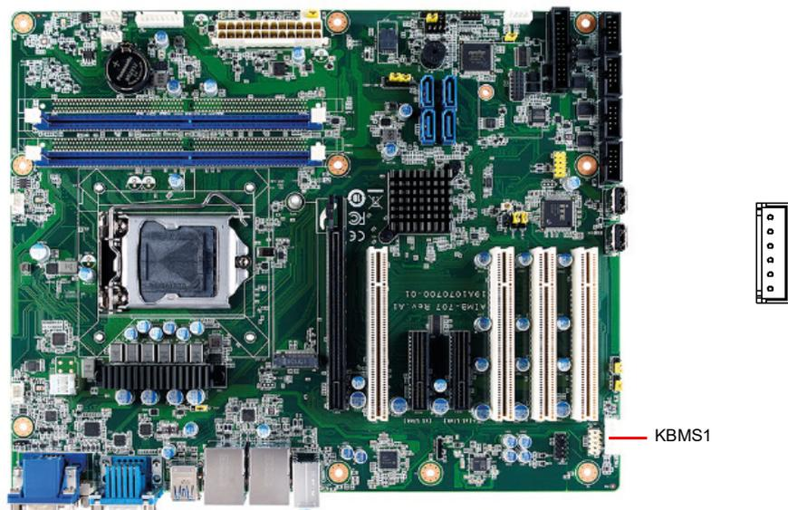
A 6-pin header (KBMS1) on the motherboard is for an optional PS/2 keyboard/mouse cable. This gives system integrators greater flexibility in designing their systems.
