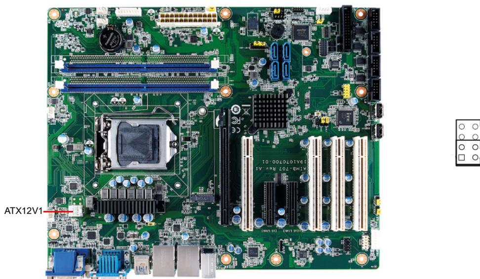
To ensure that enough power is supplied to the CPU, one auxiliary 8-pin power connector is available on the AIMB-707. ATX12V1 must be used to provide sufficient 12 V power to ensure the stable operation of the system.
