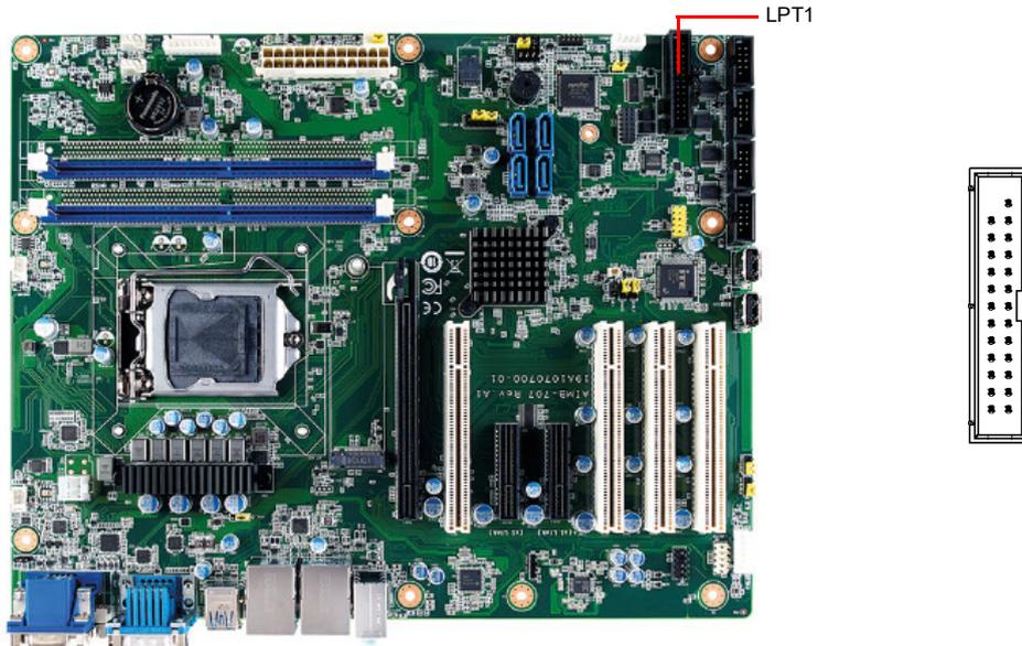
The parallel port is normally used to connect the motherboard to a printer. The AIMB-707 includes an onboard parallel port, accessed through a 25-pin flat-cable connector, LPT1.
