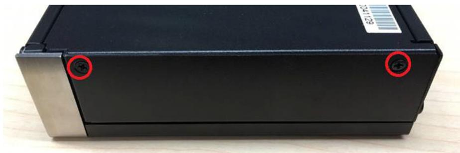
2. Unscrew the 4 screws on the HDD bay.
