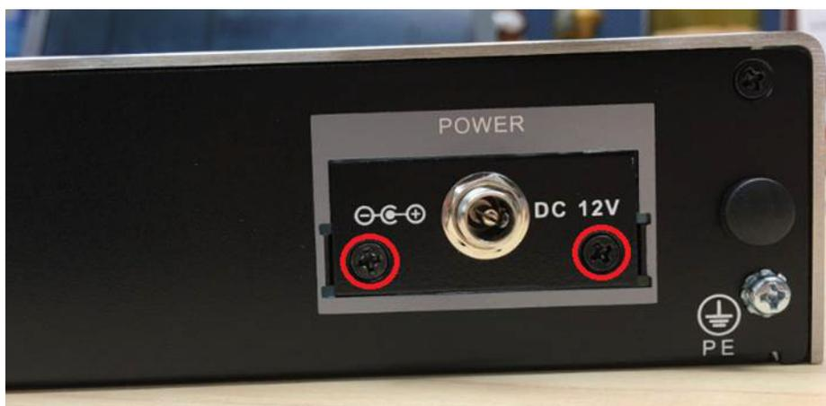
3. Unscrew the 4 screws on the bottom cover and on both sides of ARK-2230.
