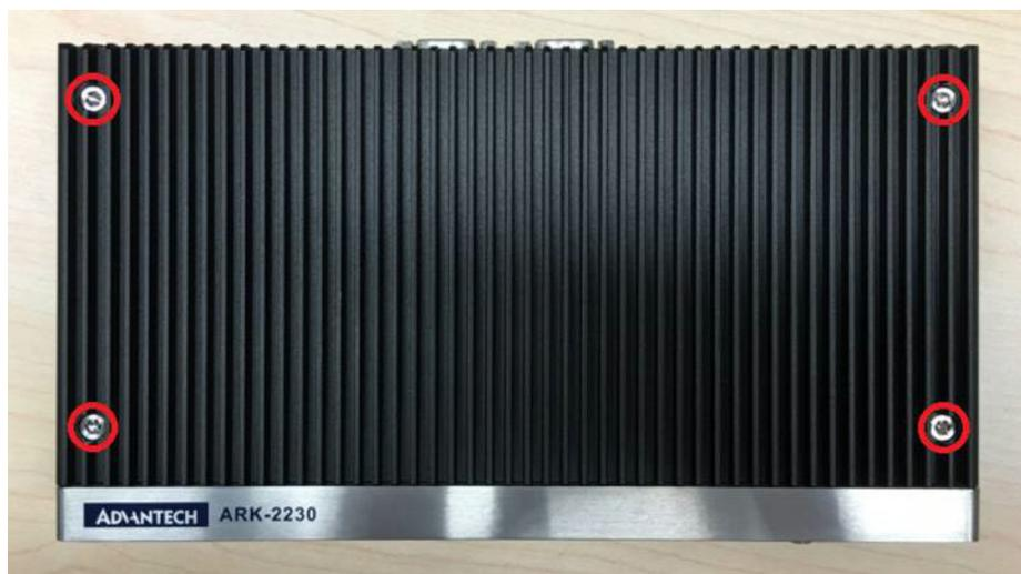
2. Remove the top cover and install the memory into the memory socket.
