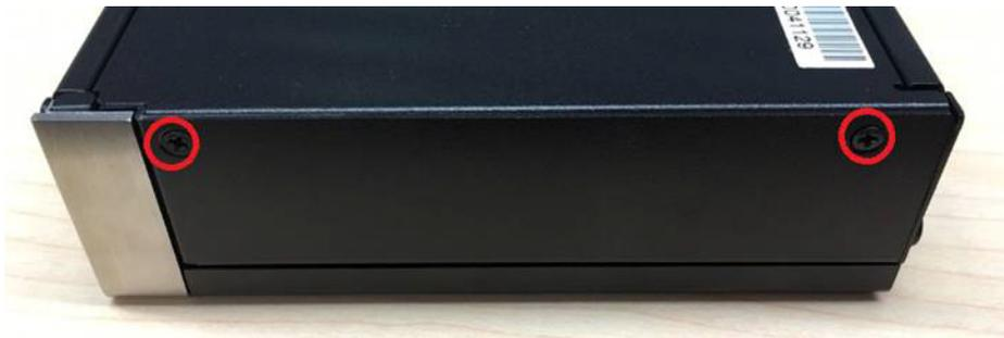
2. Put the mSATA module onto the mSATA slot (CN16), and fasten the 2 screws back on the mSATA module.
