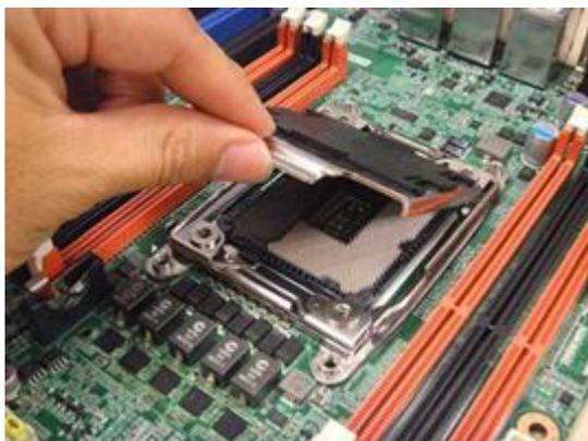
4. Position the CPU over the socket ensuring that the triangle mark on the CPU lines up with the triangle mark on the motherboard.
