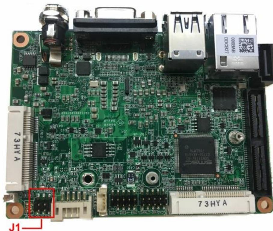
**Figure 2.1 Jumper Layout**
