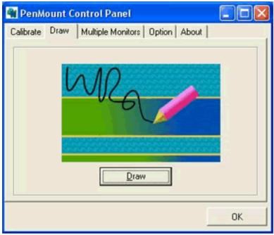
Touch the screen with your finger or a stylus and the drawing screen registers touch activity such left, right, up, down, pen up, and pen down.
