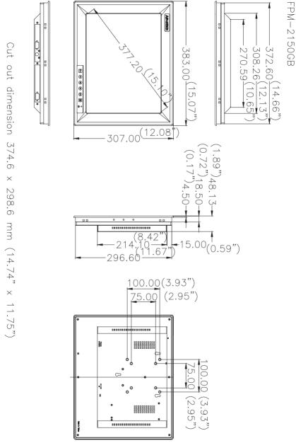
Figure 1.1: FPM-2150GB Chassis Dimensions
