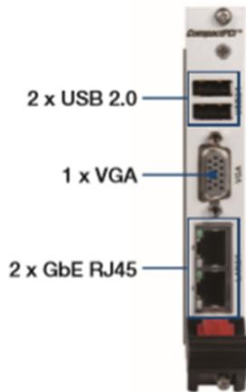
Figure 1.4 MIC-3332R1-S1E REAR IO Panel Ports and Indicators
