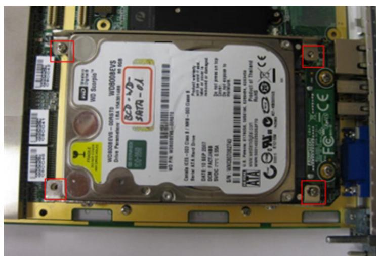
**Figure 1.6 Installing the SATA HDD into the Chassis**
