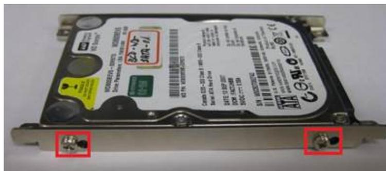
**Figure 1.5 Attach the SATA HDD to the HDD brackets**
