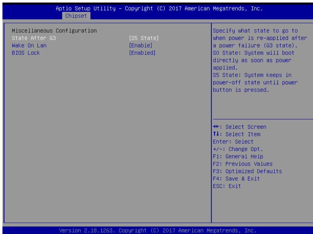
**Figure 3.36 Miscellaneous Configuration**
