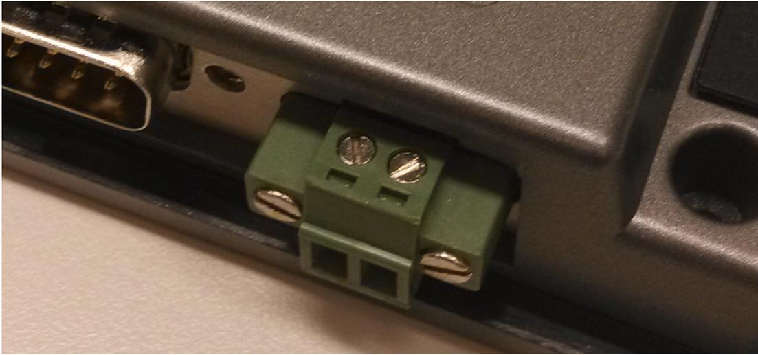
**Figure 2.3 Power Line into the Power Receptor**
