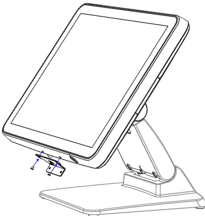
2. Connect the cables to the I/O board and fasten the screws.
