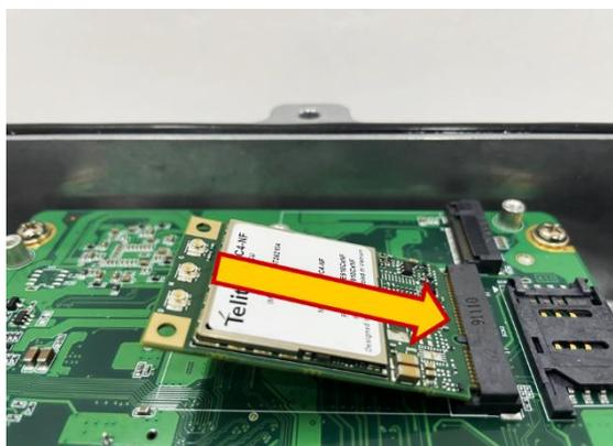
**Step 5** Press the PCI Express mini card down gently, but firmly, and then secure the card to the carrier by tightening up the one M2\*3L screw to the marked position.
