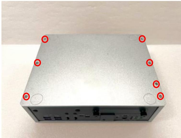
**Step 3** Remove the bottom cover, and locate the PCI Express mini card slot on the board.
