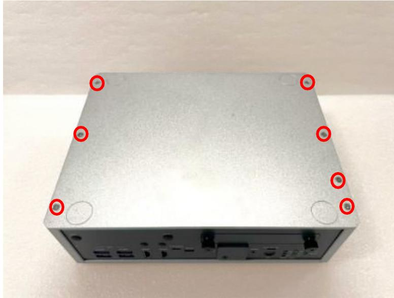
**Step 3** Remove the bottom cover, and locate the M.2 2230 Key E slot on the carrier board.
