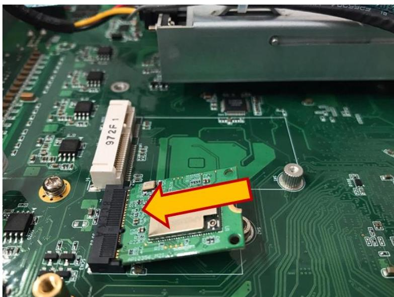
**Step 5** Press the M.2 Key E 2230 module down gently, but firmly, and then secure the module to the carrier by tightening up one M3 screw to the marked position.
