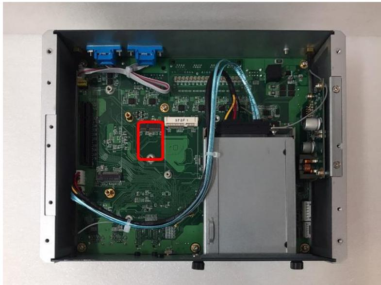
**Step 4** While holding the M.2 Key E 2230 module at a 30 degree angle up from the horizontal, slowly insert the golden fingers into the M.2 Key E 2230 slot, until it is fully inserted in place.
