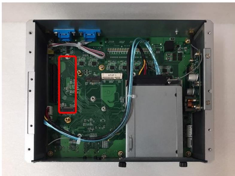
**Step 4** While holding the M.2 2280 Key M SSD drive at a 30-degree angle up from the horizontal, slowly insert the golden fingers into the M.2 2280 Key M slot, until it is fully inserted in place.
