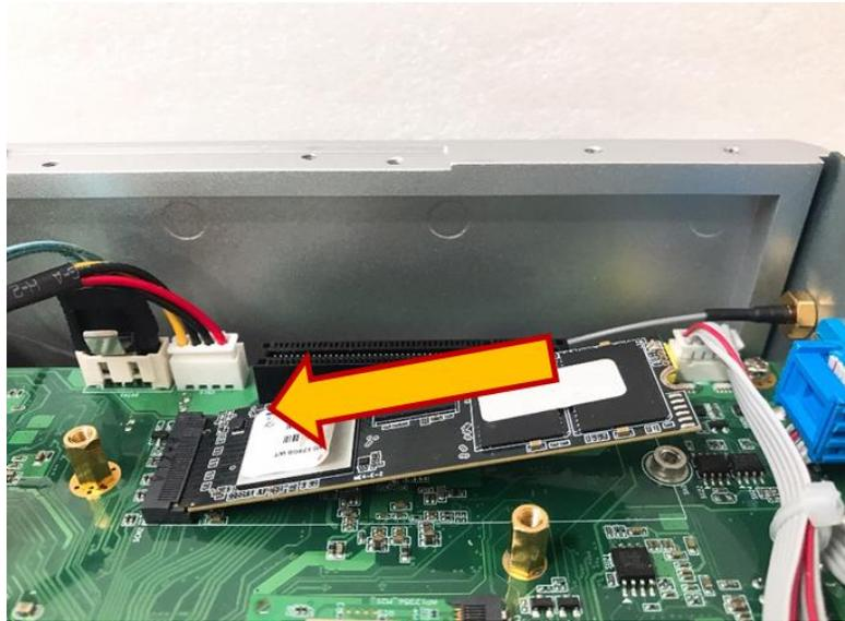
**Step 5** Press the M.2 2280 Key M SSD drive down gently, but firmly, and then secure the M.2 2280 Key M SSD drive to the carrier by tightening up one M3 screw to the marked position.
