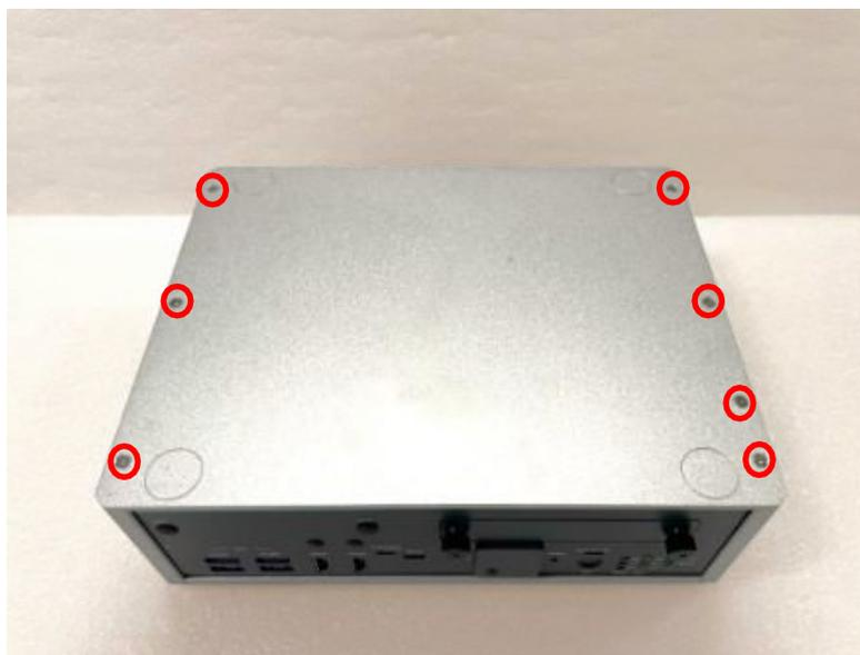
**Step 3** Remove the bottom cover, and locate the M.2 2280 Key M slot on the board.
