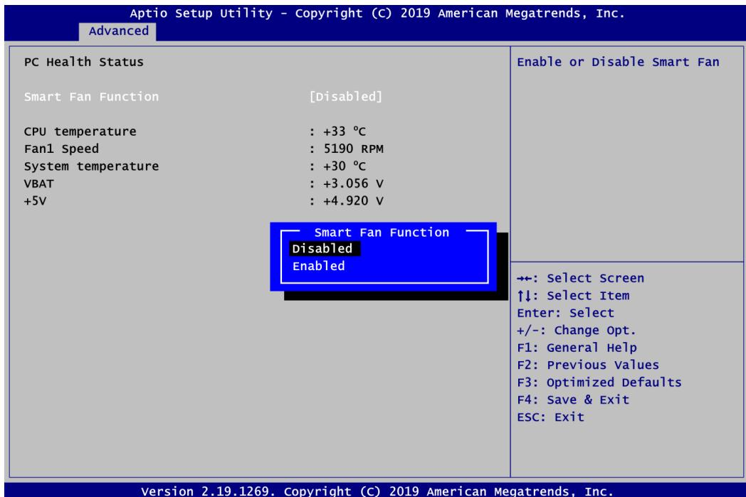
This screen displays the temperature of system and CPU, fan speed in RPM and system voltages (VBAT and +5V).
