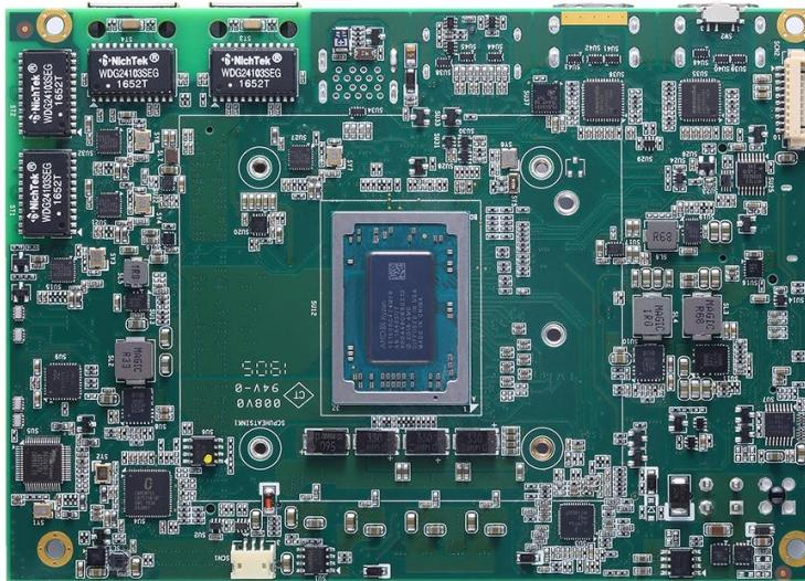
The CAPA13R, a 3.5" board, supports AMD® RYZEN® Embedded V1605B/V1807B processor. It delivers outstanding system performance through high-bandwidth interfaces, multiple I/O functions for interactive applications and various embedded computing solutions.
