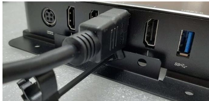
**Step 3** Fasten the tie on the HDMI cable.
