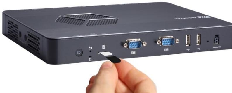
**Step 4 Complete the SIM card installation. Also use the dummy SIM card to uninstall the SIM card.**
