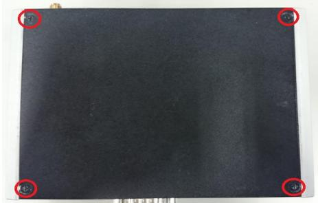
**Step 3** Please find the HDD bracket location then loosen four screws of HDD bracket to take out it.
