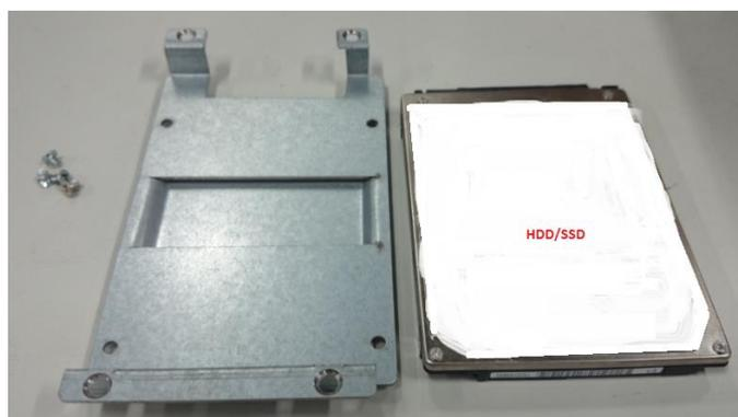
**Step 6 Fasten total four screws to fix HDD/SSD.**
