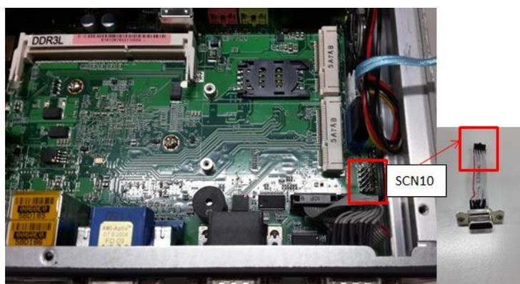
**Step 5** Please notice the high spot of connector (10 pin) then connect it into SCN10. The high spot should be faced the mini card side.
