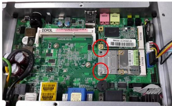
**Step 5** Assembly the bottom cover back and fasten all screws to finish installation.
