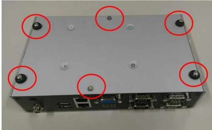
**Step 3** Remove the bottom cover and then prepare your 2.5" HDD/SSD to assemble with your bottom cover.
