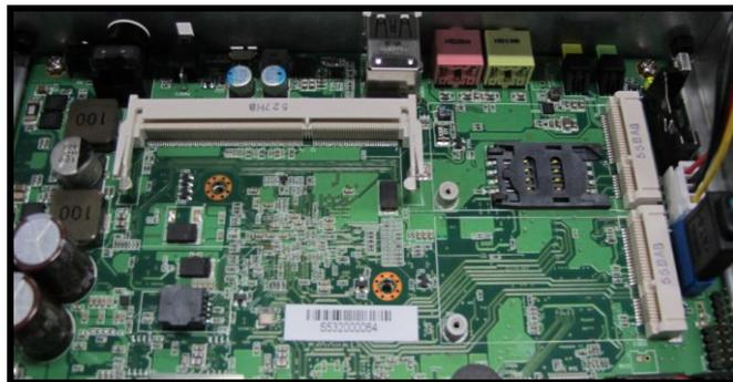
**Step 4** Slide Mini PCIe Card into Mini PCIe slot with caution and fasten screw of Express Mini Card.
