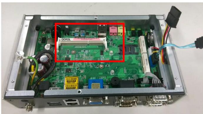
**Step 5** Locate the memory module, insert the gold colored of memory to contact into the socket.
