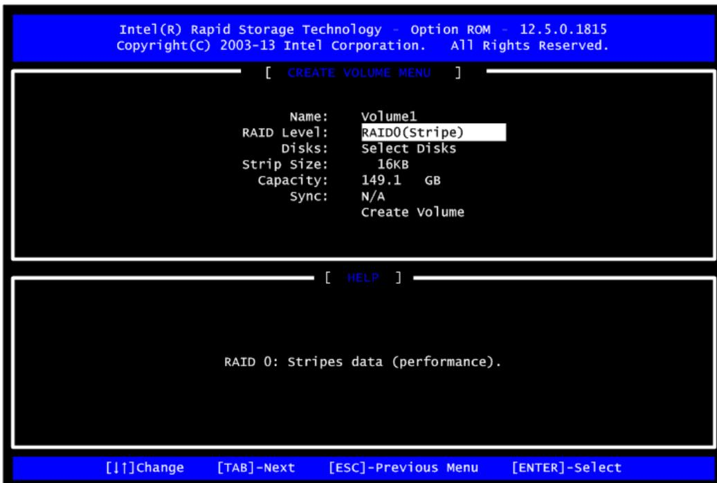
3.5. Set the stripe block size. The KB is the standard unit of stripe block size. The stripe block size can be 4KB to 128KB. After the setting, press <Enter> for the array capacity.
