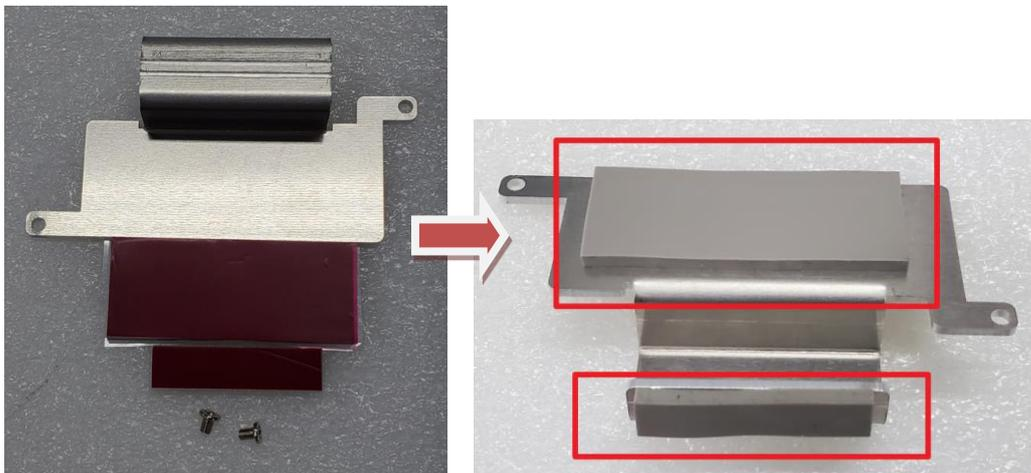
**Step 4** Insert the M.2 mini card and fasten the two screws of the bracket. Make sure the direction is correct.
