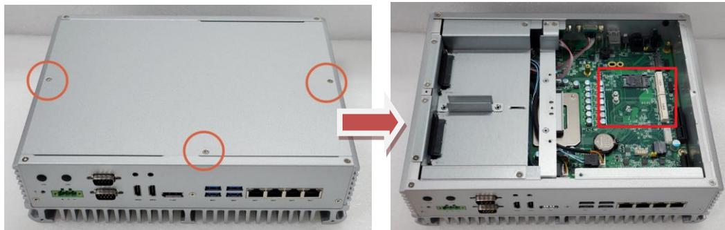
**Step 3** Insert a mini PCIe module into the sockets and then fasten the screw.
