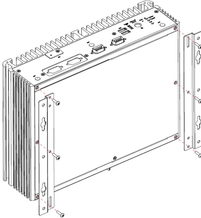
Note : If users install the screws in drywall, use the hollow wall anchors to ensure that unit does not pull away from the wall due to prolonged strain between the cable and power connector.
