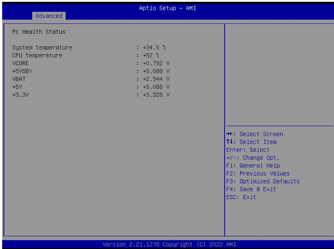
This screen displays the temperature of system and CPU as well as system voltages (VCORE, +3.3V, +5V STBY and +5V).
