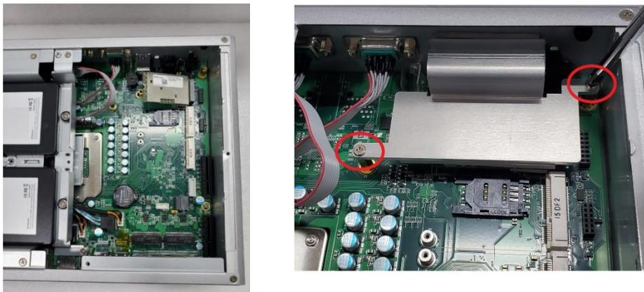
**Step 5** Put the bottom cover and fasten all screws back onto the system.
