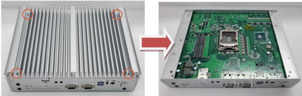
**Step 3** Remove the warning label and disengage load lever.
