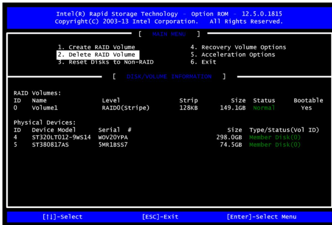
Please press <Esc> to exit the RAID BIOS utility. Now, you can proceed to install a SATA driver controller and the operating system.
