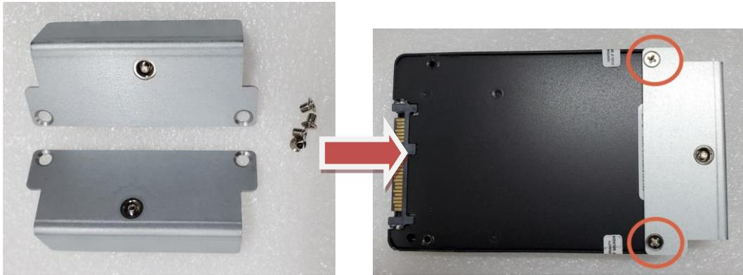
**Step 4** Push the SATA drive tray to insert the connector firmly and fasten the screw to make sure the insertion is complete.
