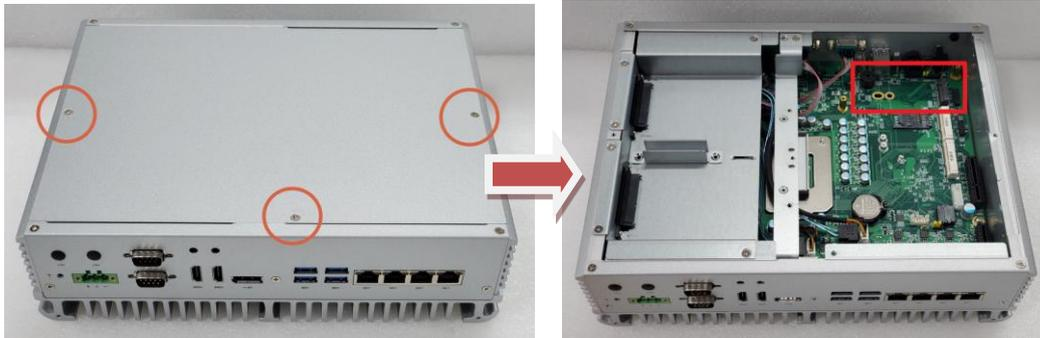
**Step 3** Please use the M.2 bracket and thermal pad from accessory, attached the thermal pad on bracket as below red marked,
