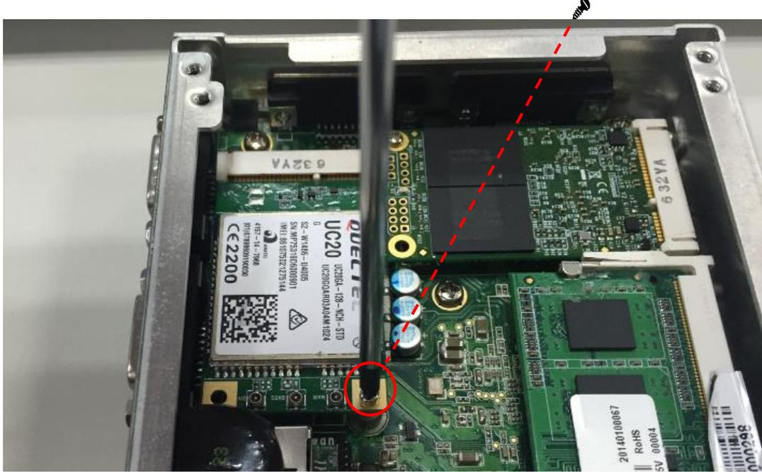
**Step6. Removing the plug cover from the chassis.**
