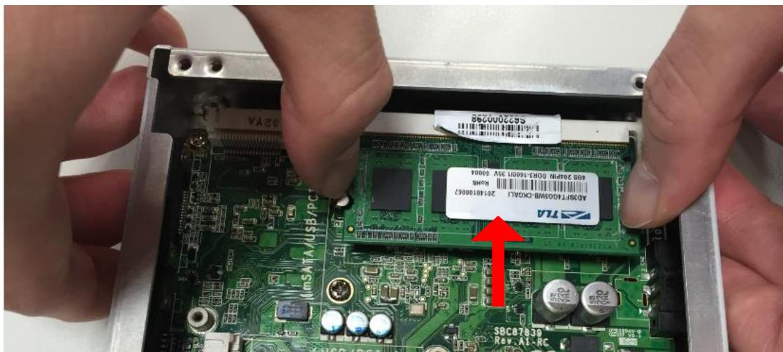
**Step 4** The memory module is locked by two latches on the sides. We strongly recommend using “LDC737” silicone on the two sides of the memory for good ability of vibration.
