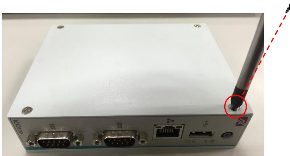
**Step3.** Following (Figure 3-1) push the SIM slot back to unlock SIM slot, inserting the SIM card and put it back(Figure 3-2), and lock the SIM slot(Figure 3-3).
