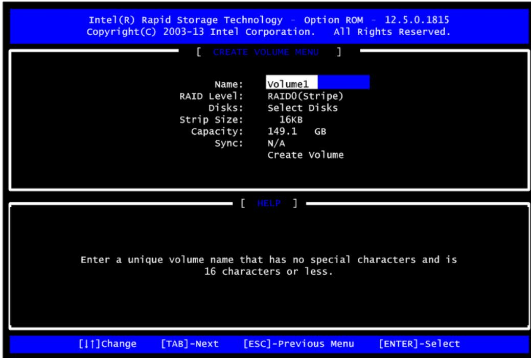
3.4. When finished, press <Enter> to select a RAID level. There are four RAID levels: RAID0, RAID1, RAID5 and RAID10. Select a RAID level and press <Enter>.
