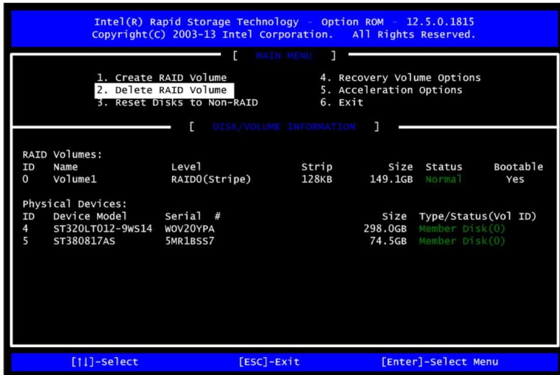
Press <Esc> to exit the RAID BIOS utility. Now, you can proceed to install a SATA driver controller and the operating system.
