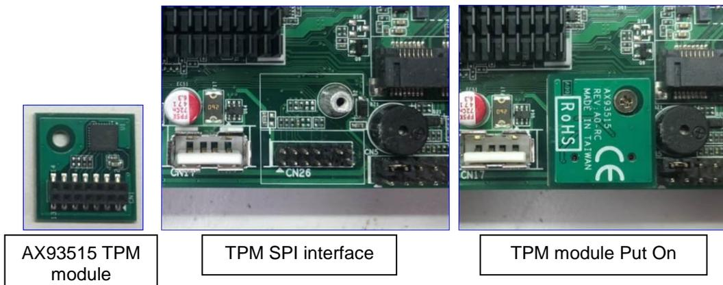
2. There are two ways to confirm whether the TPM Module is installed successfully or not:
