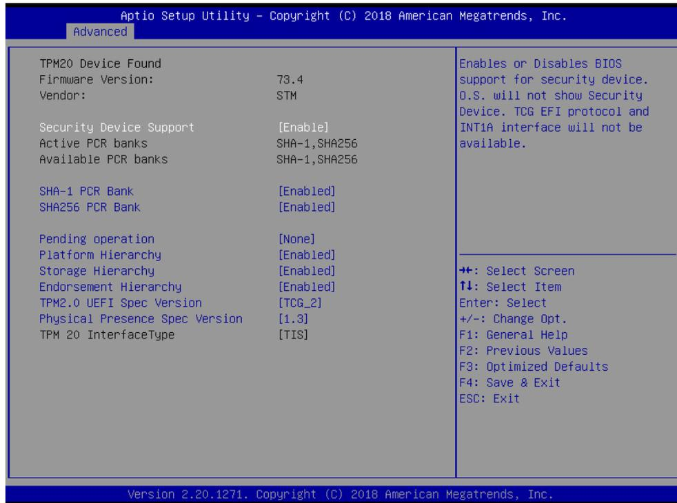
(In the Trusted Computing section, on the first of line will show "TPM2.0 Device Found", if installation is successful.)
