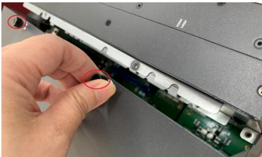
**Step 4** Locate the PCI or PCIe slots which you want to add the card in, and remove the holder bracket and slot bracket.
