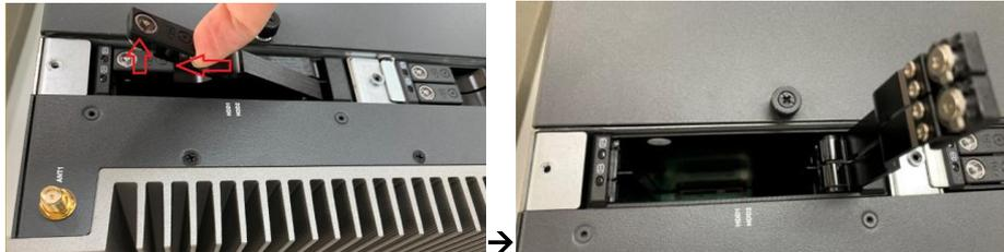
**Step 5** Insert the HDD into the HDD tray.
