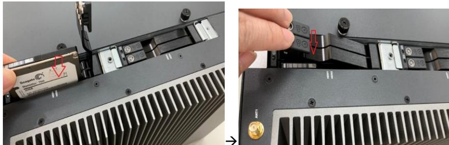
**Step 6** Screw the bracket. The installation is complete.
