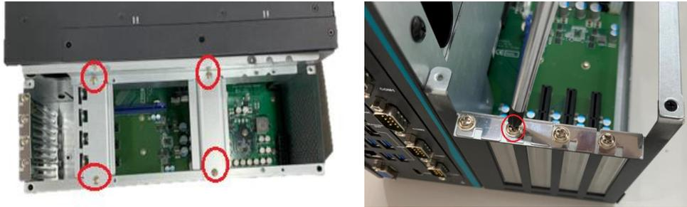
**Step 5** Align the PCI or PCIe card with the slot, press the card into the slot until it is firmly seated and screw it.
