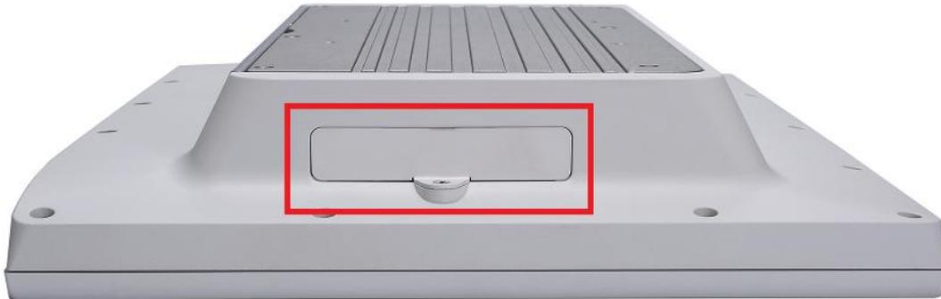
**Step 3** Locate the CFast™ socket, and insert the card into the socket.
