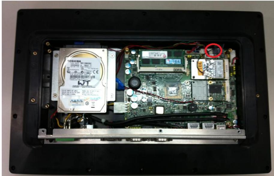
**Step 4 There are two connectors on wireless LAN card. One is MAIN, and the other is auxiliary. Connect antenna cable to MAIN connector on wireless LAN card.**
