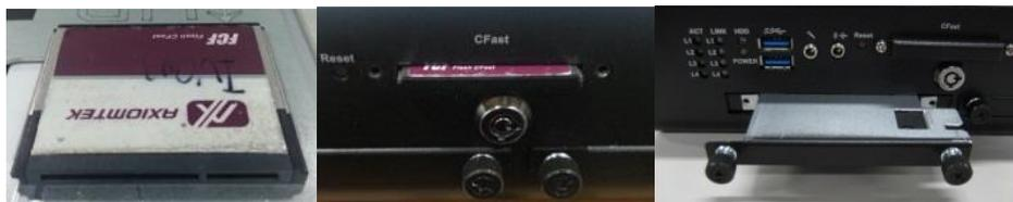
**Step 4** Secure CFast and SATA drive to complete the installation.
