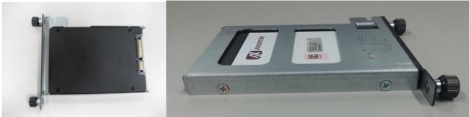
**Step 3** Install CFast and SATA drive to the slot.
