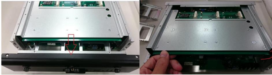
**Step 7 Loosen below screws to remove cover and put on the thermal pad.**
