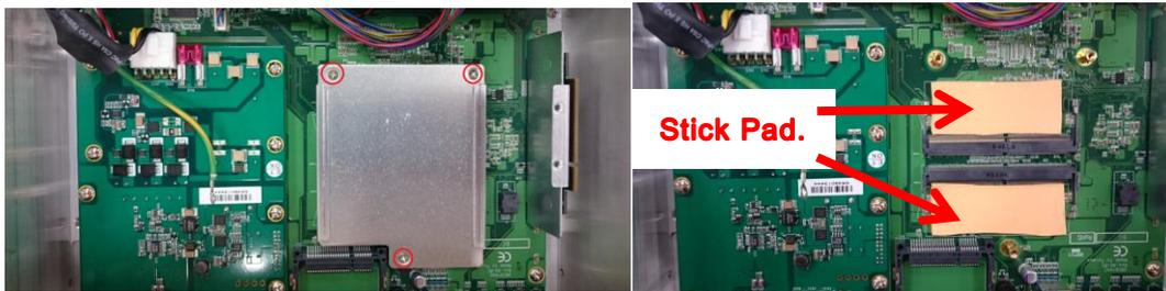
**Step 8 Install the DDR cautiously and put on the thermal again.**
