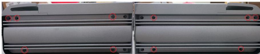
**Step 6 Pull out the front bezel and internal bracket as shown.**
