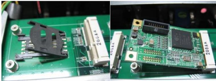
Step 4 Fasten the screws to complete the installation.
