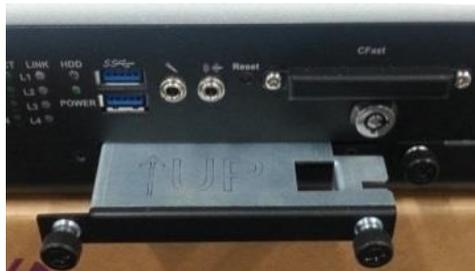
**Step 2** Slide HDD into the cover as picture shown. Insert screws into each side of the SATA drive through the corresponding holes.
