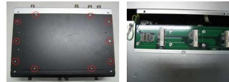
**Step 2** Install the SIM card or Mini PCIe module and fasten screws. Notice the signal support type of the mini card slot when installing the card. Fasten screws.
