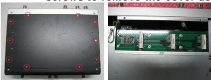
**Step 2** Loosen the lateral screws as shown.
