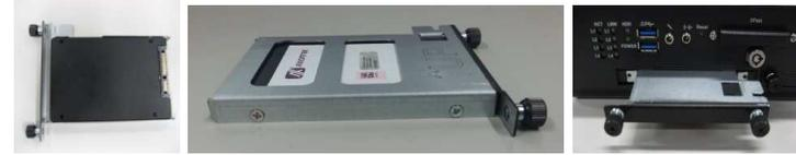
**Step 3** Insert the SATA drive and then the CFast into their slots respectively, as shown in the pictures
