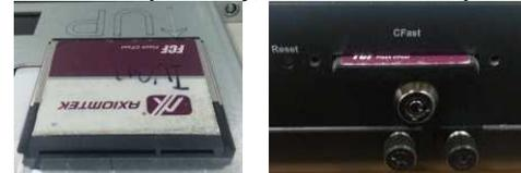
**Step 4** Secure CFast and SATA drive by fastening all of the screws tightly to complete the installation.
