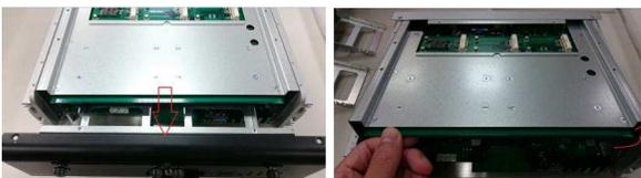
**Step 4** Remove the DRAM cover by loosening the screws. Install DRAM and then stick the thermal pad on it.
