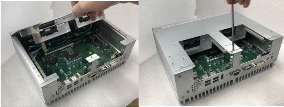
**Step 7** Slide the secured SATA tray back and fasten screws tight to complete the installation.
