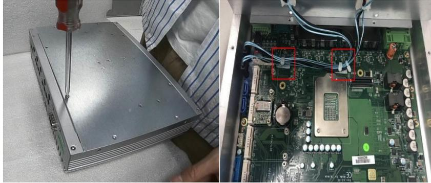
**Step 4** Insert the wireless module (3G/4G/BT/GPS module etc.) into the slot with the marking "PCIe / USB". Then fasten the screws as shown.
