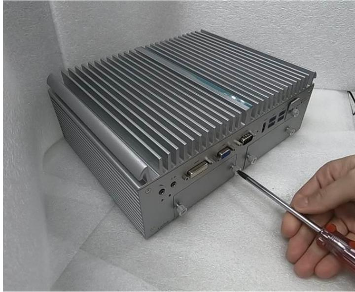
Step 3 Extract the SATA drive tray. Each drive tray can install two storage drives.
