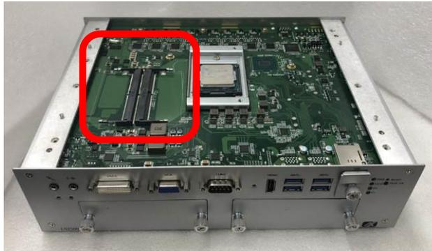
**Step 4** Insert the gold colored contact of the memory module into the socket and push the module's two end latches down until locked.
