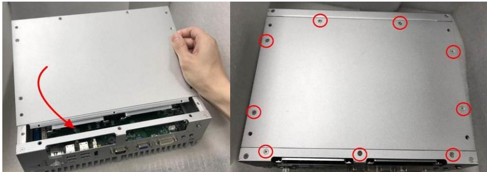
**Step 7** Slide the SATA trays back and fasten screws firmly to complete the installation.
