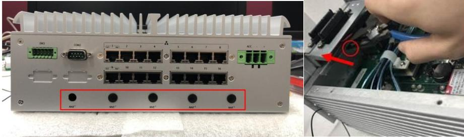
**Step 8 Connect the RF cable to the connector of the 3G module marked with "MAIN".**
