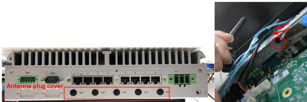
**Step 6** Connect the RF cable to the connector of the 3G module marked with "MAIN".
