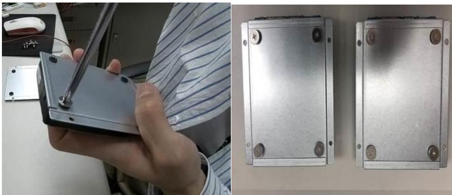
**Step 5** Put the drive holders to precisely meet the screws hole positions and tighten screws.
