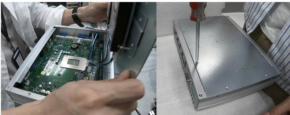
**Step 11 Flip over the system, and screw the RF antenna tight.**
