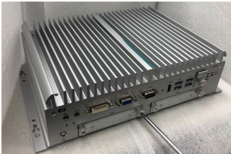
**Step 3** Extract the SATA drive tray. One drive tray can install two SSD/HDD drives.
