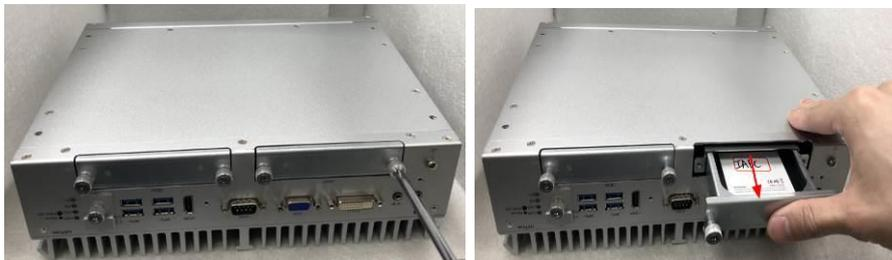
**Step 4** Loosen all screws and open the bottom cover carefully.
