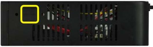
Figure 15: USB Knockout Holes
