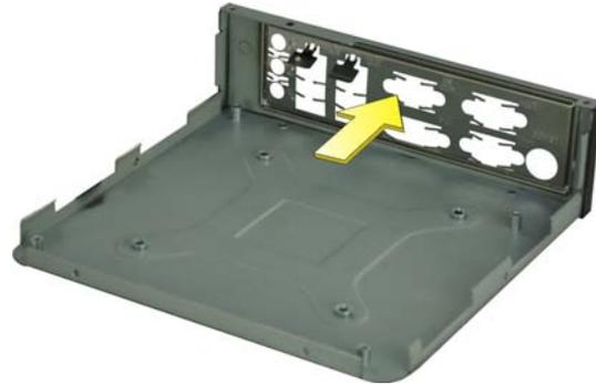
Figure 3: I/O Shielding Installation
