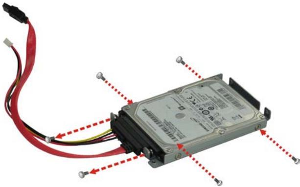
Figure 6: HDD Retention Screws
