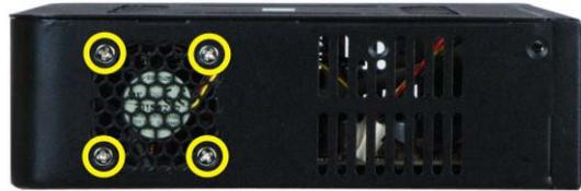
Figure 14: System Fan Retention Screws
