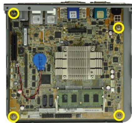
Figure 4: Motherboard Retention Screws
