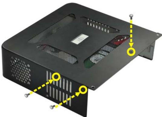
Figure 7: HDD Installation
