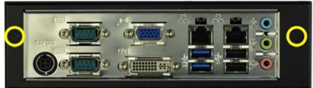
Figure 8: Knockout Holes for Wireless Antenna
