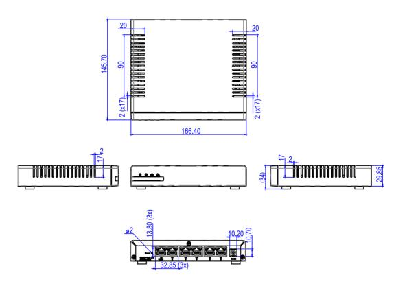
Figure 1-4: Physical Dimensions (millimeters)
