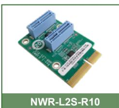
The outwards-facing riser card (P/N: NWR-L2S-R10), although lower in height, is able to provide better spacing to ensure expansion cards run at a low temperature. It is ideal for the chassis that is wide enough for the expansion card to be placed.
