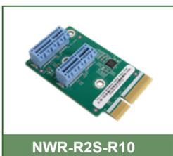
The inwards-facing riser card (P/N: NWR-R2S-R10) is designed with higher height to keep a decent space between the expansion cards and the motherboard. This can help improve the airflow and heat transfer within the system. It is suitable for installation where space is limited. Moreover.
