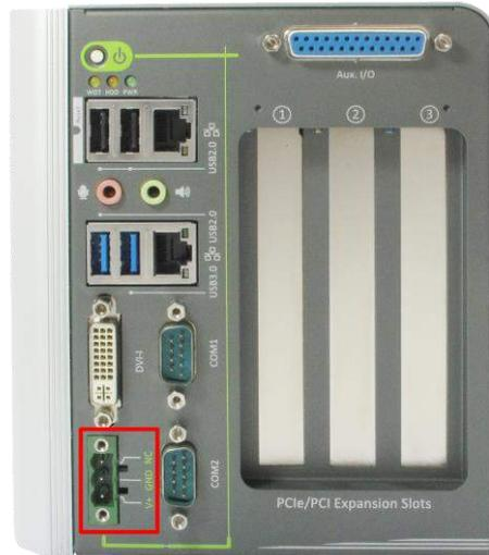
Figure 9: DC-input connector
