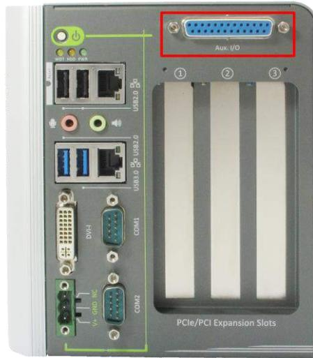
Figure 10: Isolated DI/O connector
