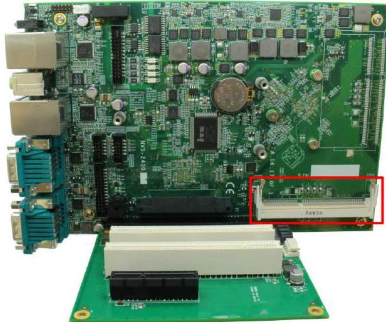
Figure 15: DDR3L SODIMM socket
