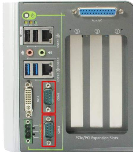
Figure 6: Software-programmable COM ports
