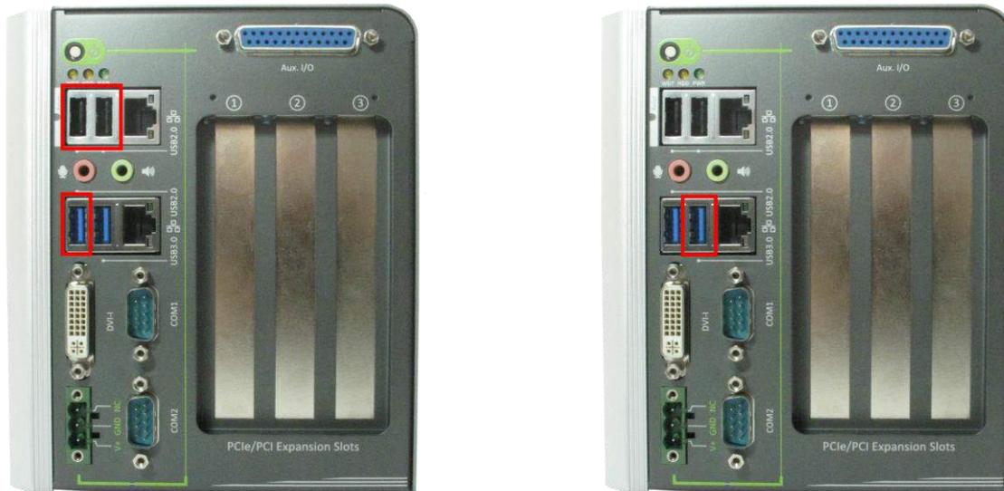
Figure 7: USB2.0 connectors (left) and USB3.0 connector (right)
