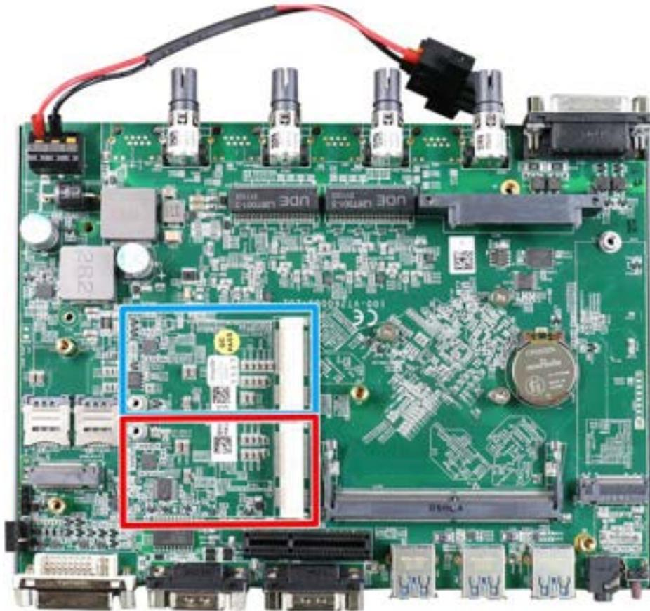
1. To install the mini PCIe module, insert the module on a 45° angle and secure the module using the screw provided.
