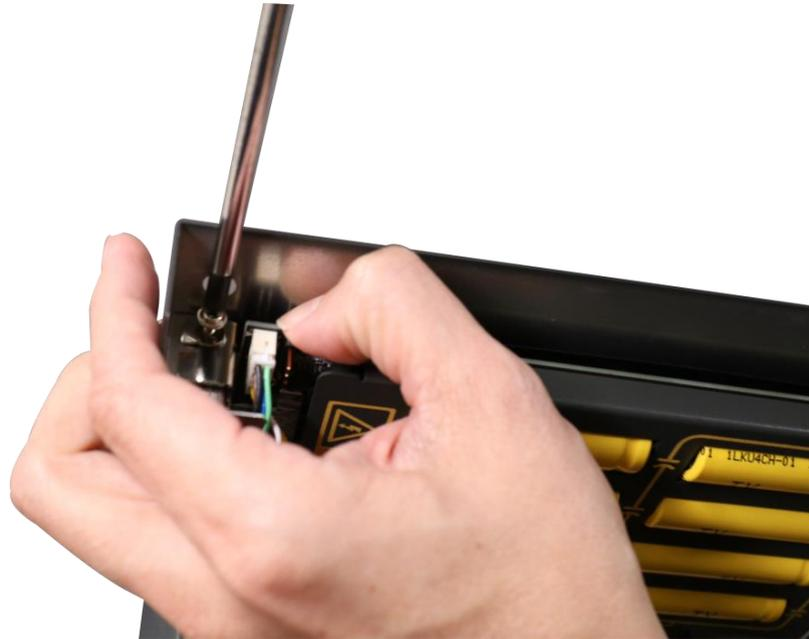
9. Once the PCIe add-on card has been installed, place the L-shaped cover back onto the Cassette module and secure the screw indicated.
