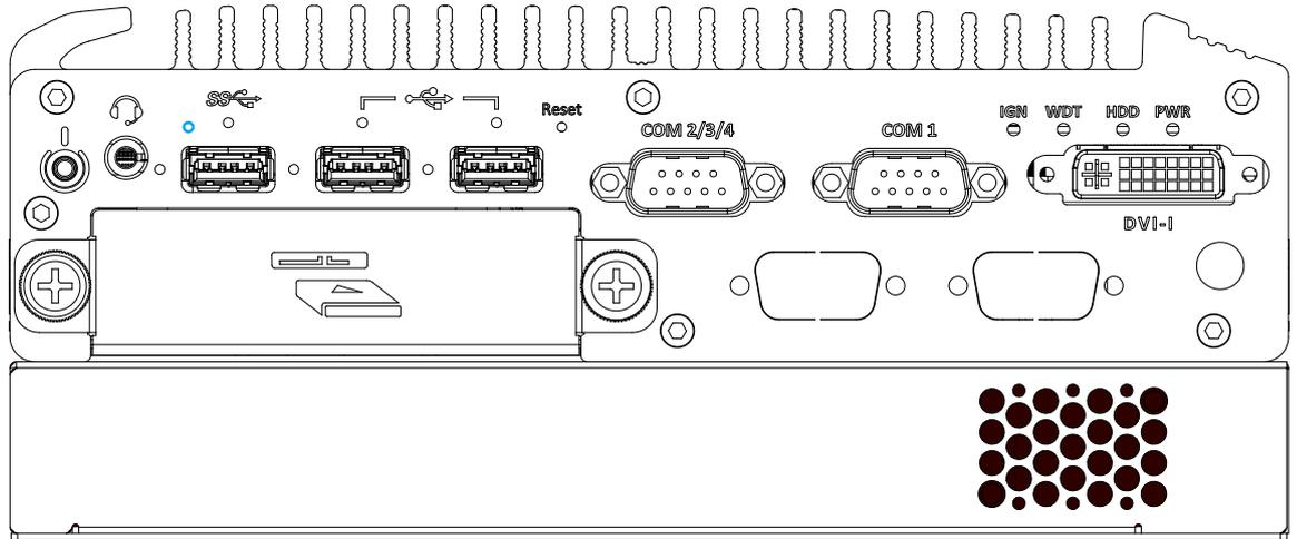
The CMOS Reset button is used to manually reset the motherboard BIOS in case of system halt or malfunction. To avoid unexpected operation, it is purposely placed behind the panel. To reset, please use the tip of a pen, press and hold for at least 5 seconds to reset the BIOS.
