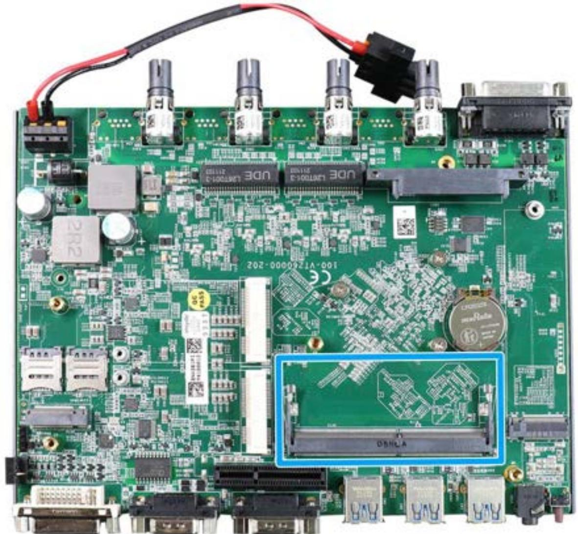
The system motherboard supports a SODIMM socket for installing a DDR4-3200 memory module up to 32GB capacity.
