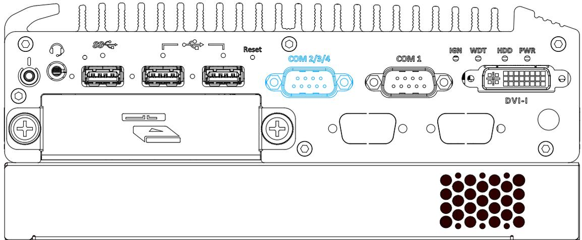
Implemented using industrial-grade ITE8786 Super IO chip (-40 to 85°C) and provide up to 921600 bps baud rate, the second D-Sub male connector (COM2/ 3/ 4) can be configured in BIOS as single RS-422/ 485 port (COM2) or three 3-wire RS-232 ports (COM2/COM3/COM4). Please refer to [COM2/ 3/ 4 Port Configuration](#) for configuring operation mode. An optional 1-to-3 Y-cable is available to connect three RS-232 devices.
