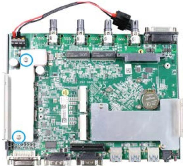
3. Remove the heatsink to access the M.2 3042/ 3052 B key and SIM card slots.
