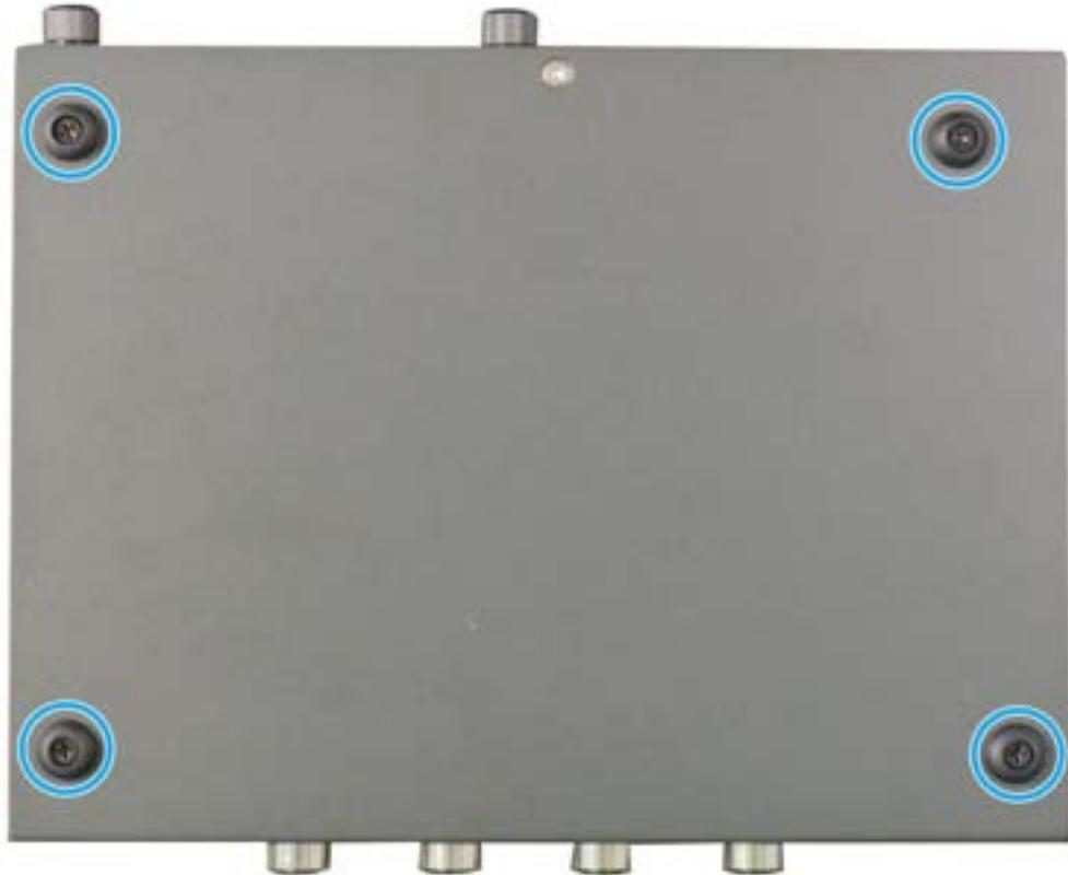
2. Take the **damping bracket** out of the accessory box, insert four **anti-vibration grommets** into the location shown on the bracket, and secure the bracket onto the bottom of the enclosure using four **M4 screws**.
