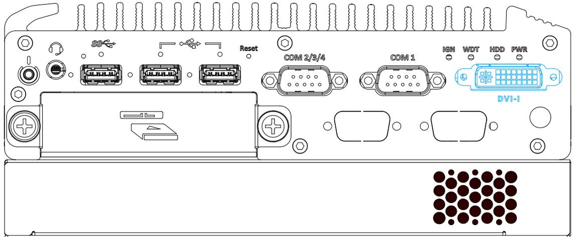
The system features a DVI-I connector on its front panel that is also compatible with VGA signals. The DVI and VGA outputs are directly driven by integrated Intel HD graphics engine and support up to 1920 x 1080 resolution.
