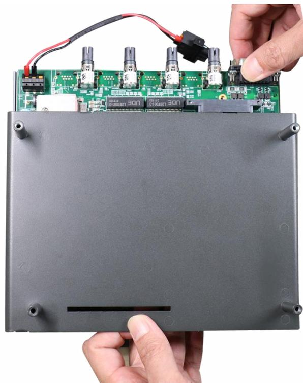
3. Plug in the 3-pin connector and use a small Phillips screwdriver to secure the connector.
