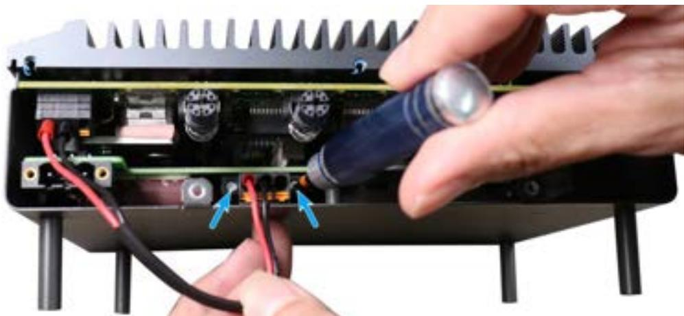
Release screws on the 3-pin connector
