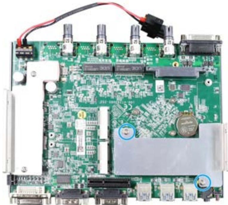
2. Remove the heatsink to locate the SODIMM memory module slot on the motherboard.
