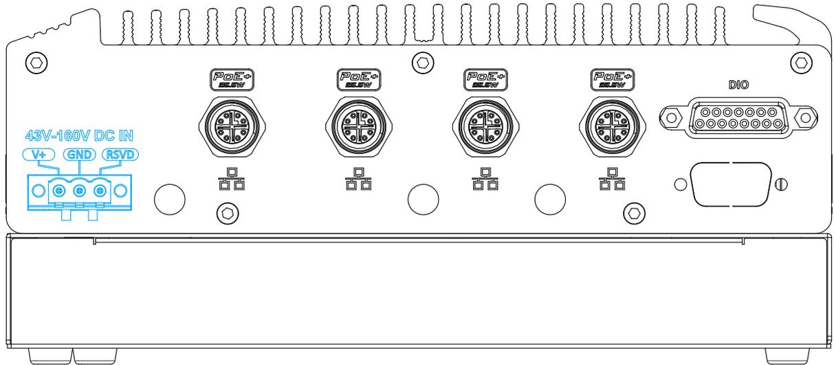
The system accepts a wide range of DC power input from 43V to 160V via a 3-pin pluggable terminal block, which is fit for field usage where DC power is usually provided. The screw clamping mechanism on the terminal block offers connection reliability when wiring DC power.
