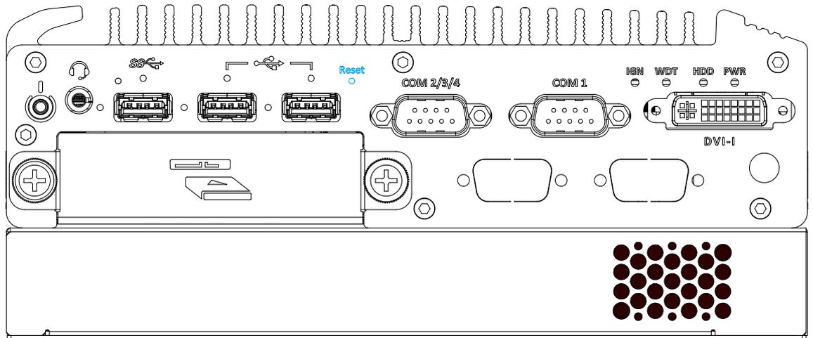
The reset button can be used to manually reset the system in case of abnormal condition. To avoid unexpected operation, the reset button is hidden behind the front panel. You need to use a pin-like object to push the reset button.
