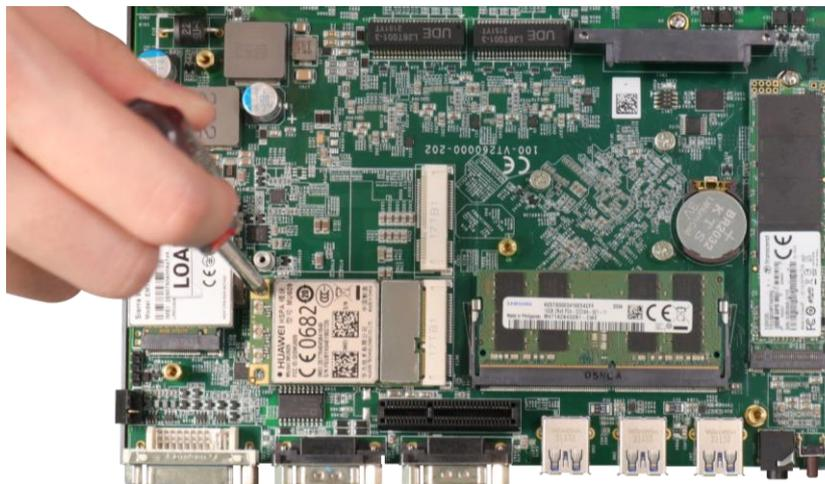
Insert on a 45° angle and secure using the screw provided
