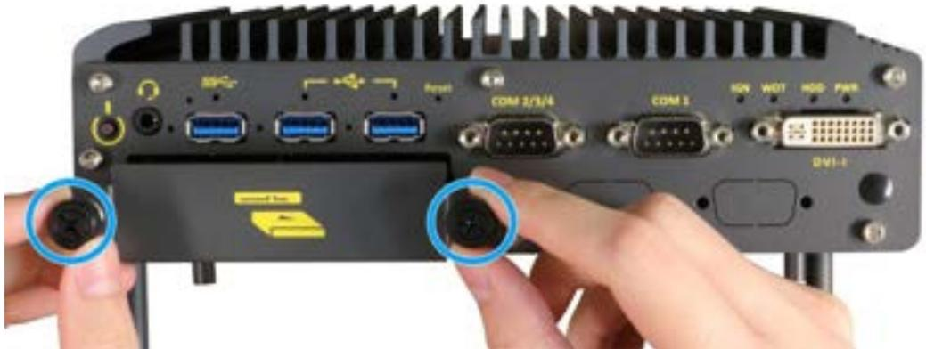
2. Gently pull out the 2.5” HDD/SSD tray. With HDD/SSD label downwards, secure the HDD/ SSD using the screws provided (indicated in blue), there are two screws on each side.
