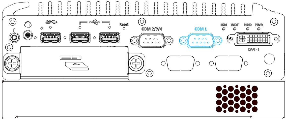
Isolated with up to 15kV ESD protection, the port is implemented using industrial-grade ITE8786 Super IO chip (-40 to 85°C) and provides up to 921600 bps baud rate. COM1 is aRS-485 port via 9-pin D-Sub male connector. The following table describes the pin definition of COM ports.
