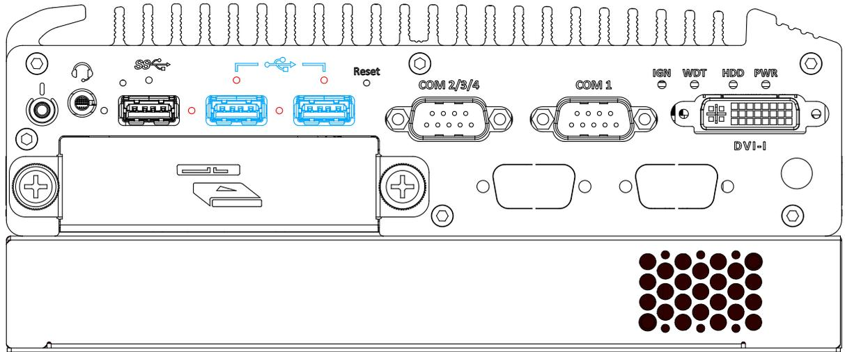
The system offers two USB2.0 ports on its front panel with screw-lock mechanism (indicated in red). They are backward-compatible with USB 1.1 and USB 1.0 devices. Legacy USB support is also provided so you can use USB keyboard/mouse in DOS environment.
