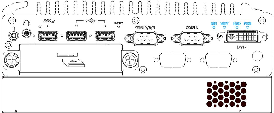
There are four LED indicators on the I/O panel: PWR, WDT, HDD and IGN. The descriptions of these LEDs are listed in the following table.
