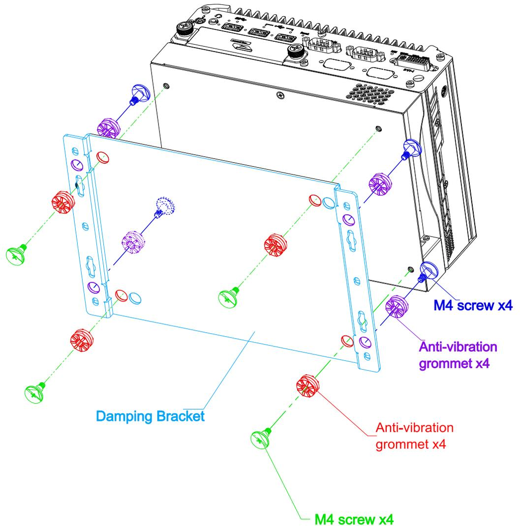
3. Referring to the illustration shown above, insert four **anti-vibration grommets** into locations on the side hinges indicated, secure the system using four **M4 screws** onto a flat surface in the vehicle.
