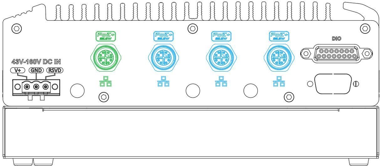
The system offers four PoE+ GbE ports via M12 X-coded connectors on the front panel. The ports are implemented using Intel® I210 controller and the port indicated in **green** supports Wake-on-LAN.
