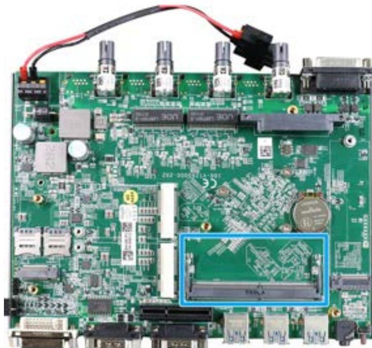
3. To install the memory module, insert gold fingers of the module into the slot at 45 degree angle, push down on the edge of the module and the clips on the side should clip the module into position.
