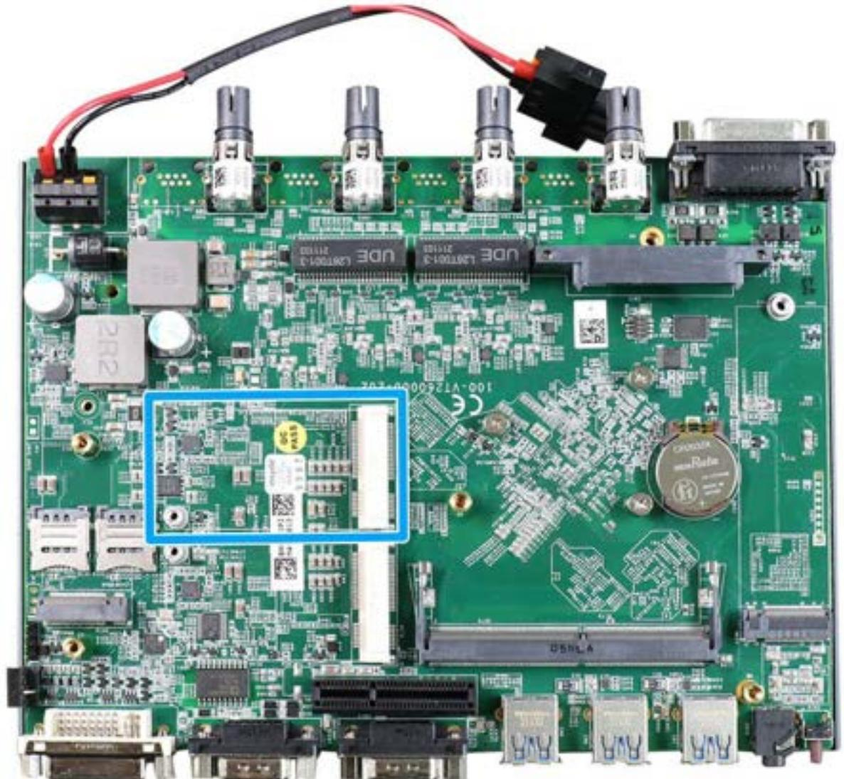
There is a full-size USB2.0 signal only mini-PCle socket for better compatibility with off-the-shelf mini-PCle wireless modules. For customers who want to install a mini-PCle wireless module, please take advantage of the mini-PCle socket and the antenna openings on the panels.
