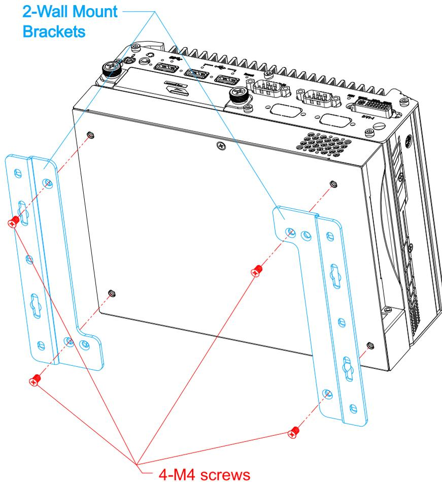
3. Place the system on a flat surface portion of the wall and secure it with four (4) M4 pan screws.
