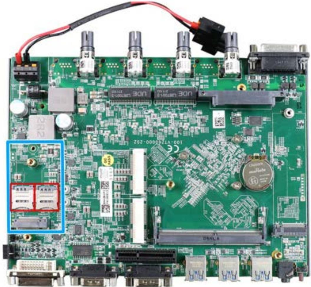
The system has one M.2 3042/ 3052 B key socket (in blue) for 5G/4G module installation and dual SIM slots (in red). The M.2 slot features USB3.1 and USB 2.0 signal.
