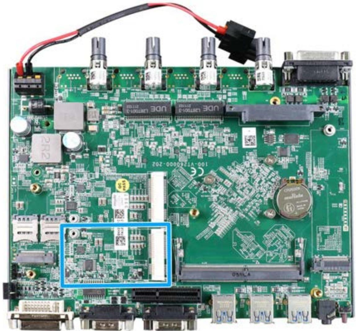
The mini-PCIe socket (in blue) accepts off-the-shelf mini-PCIe modules. You can add additional features to your system such as 5G/ 4G, WiFi, GPS, CAN bus, analog frame grabber, etc.
