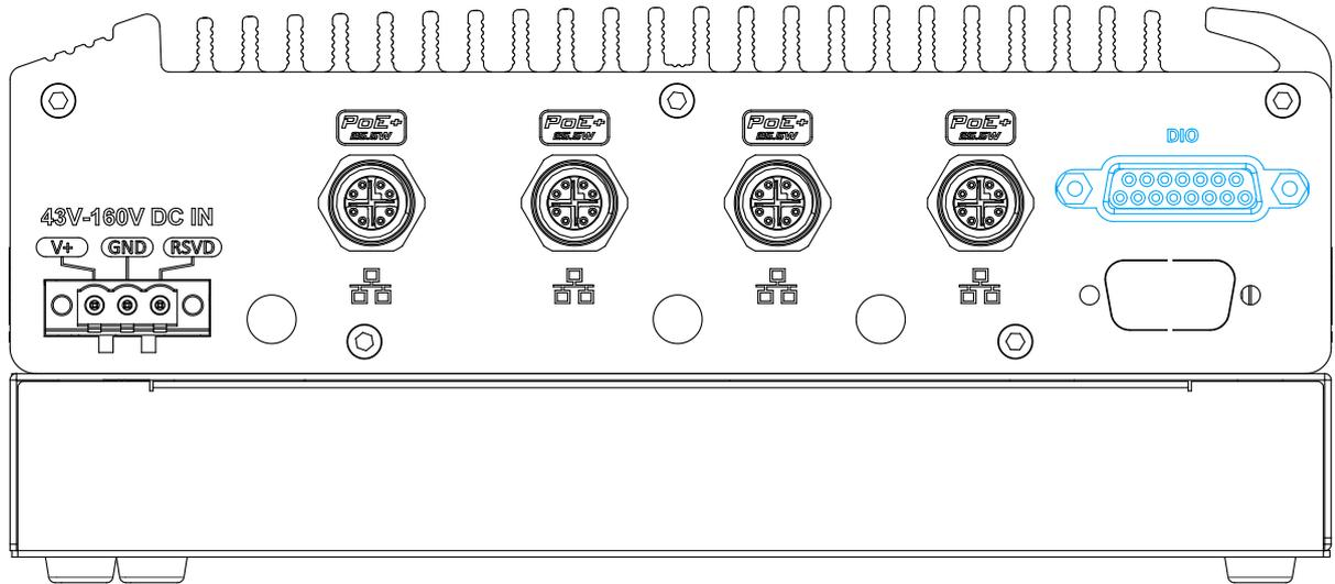
The system provides 4x isolated digital input channels and 4x isolated digital output channels. The DIO functions support polling mode I/O access and DI change-of-state interrupt. Please refer to [Watchdog Timer & Isolated DIO](#) for information on wiring and programming the isolated DIO channels.
