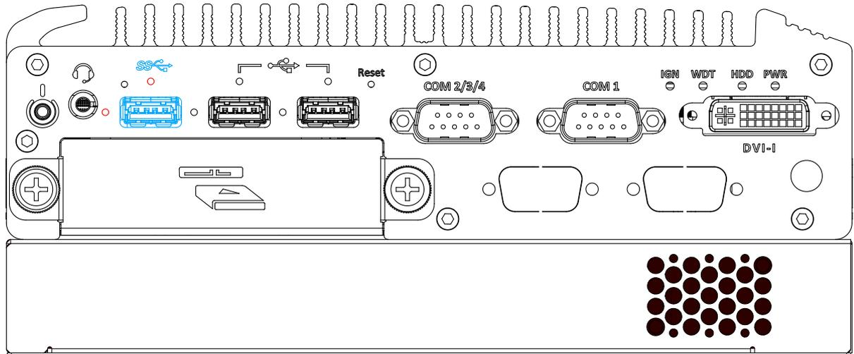
The system offers one USB3.1 Gen1 (SuperSpeed USB) port on its front panel with screw-lock mechanism (indicated in **red**). It is backward-compatible with USB 2.0, USB 1.1 and USB 1.0 devices. Legacy USB support is also provided so you can use USB keyboard/mouse in DOS environment while USB 3.1 Gen1 driver is supported natively in Windows 10.
