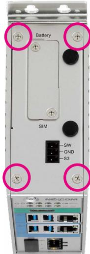
2. Remove the screws on the bottom chassis.
