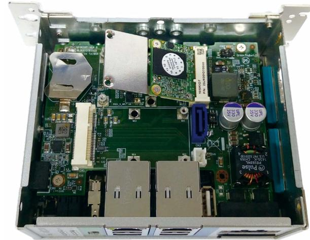
3. When installing a 3G module, make sure to install the SIM card first.
