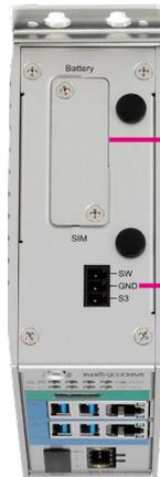
RTC Battery Socket
