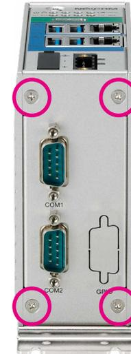
3. Remove the screws on the rear chassis.
