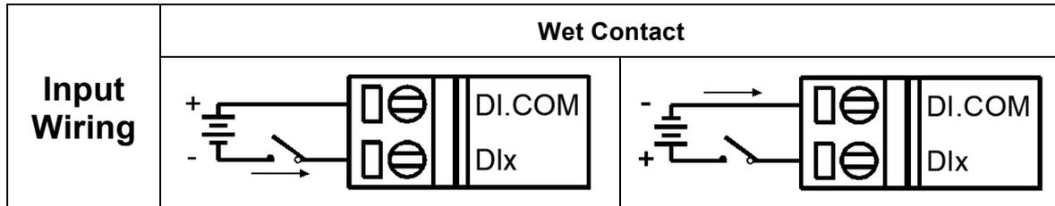
Figure 12 DI electrical wiring diagram
