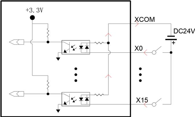
Figure 7 DI PNP wiring solution
