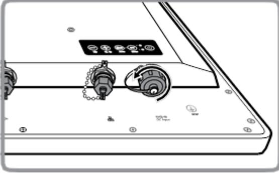
2. Plug the AC adapter to the DC-in jack of your device. Make sure the cable fits to the connector, then tighten the O-ring (by turning it clockwise) to secure the connection.
