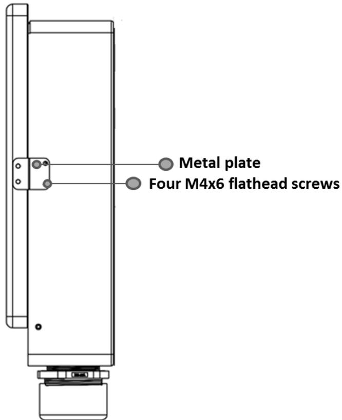
**Step 6** Carefully mount the device to the fixture (for ex. wall).
