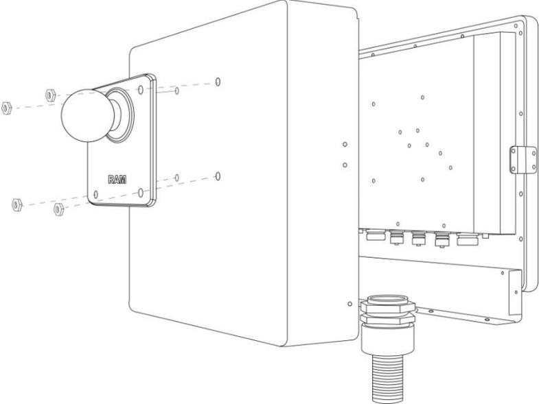
A line drawing of the enclosure with the top cover reattached. A VESA mounting plate is mounted on the front of the enclosure. Four metal nuts are shown being inserted from the outside of the enclosure into the VESA plate. Dashed lines indicate the path of the nuts through the enclosure's front panel and into the VESA plate. A RAM module is visible inside the enclosure, and a connector is shown at the bottom. |
